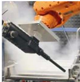
Figure 1-2: Examples for surface inspection and treatment technologies. (left): mobile FT-IR instrument; (right): automated CO 2 snow cleaning
